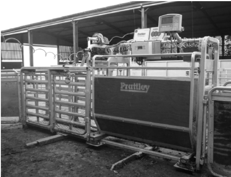
Figure 3. The Pratley autodrafter unit fitted with a TruTest XR3000 in the handling unit at Didling farms.
