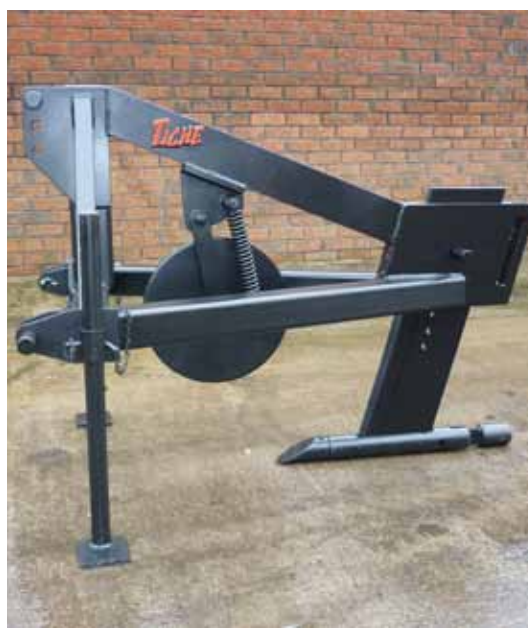
Figure 3. Mole plough showing cylindrical foot and expander
